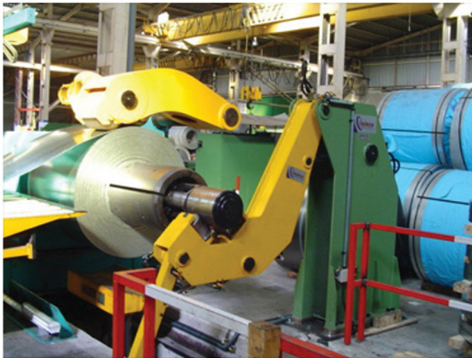
7.- Support for cantilever mandrel for coils up to 20 t. weight
