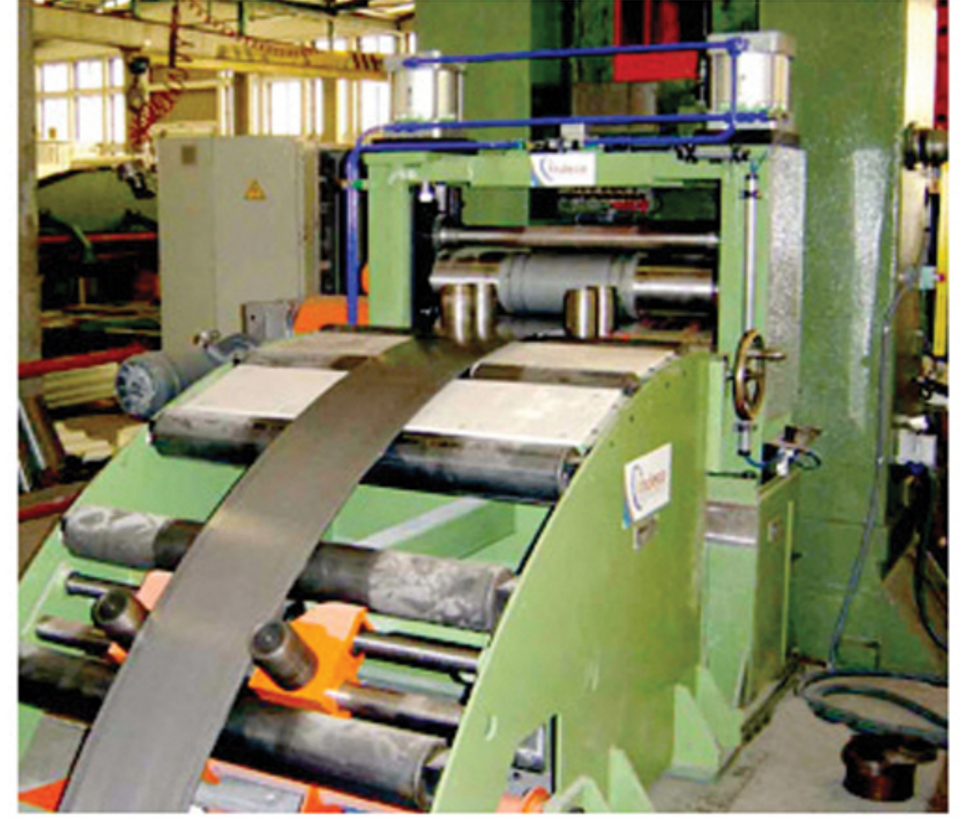
4.- Feeder Rolls with vertical strip guides for strip of 3 mm. x 600 mm width.
