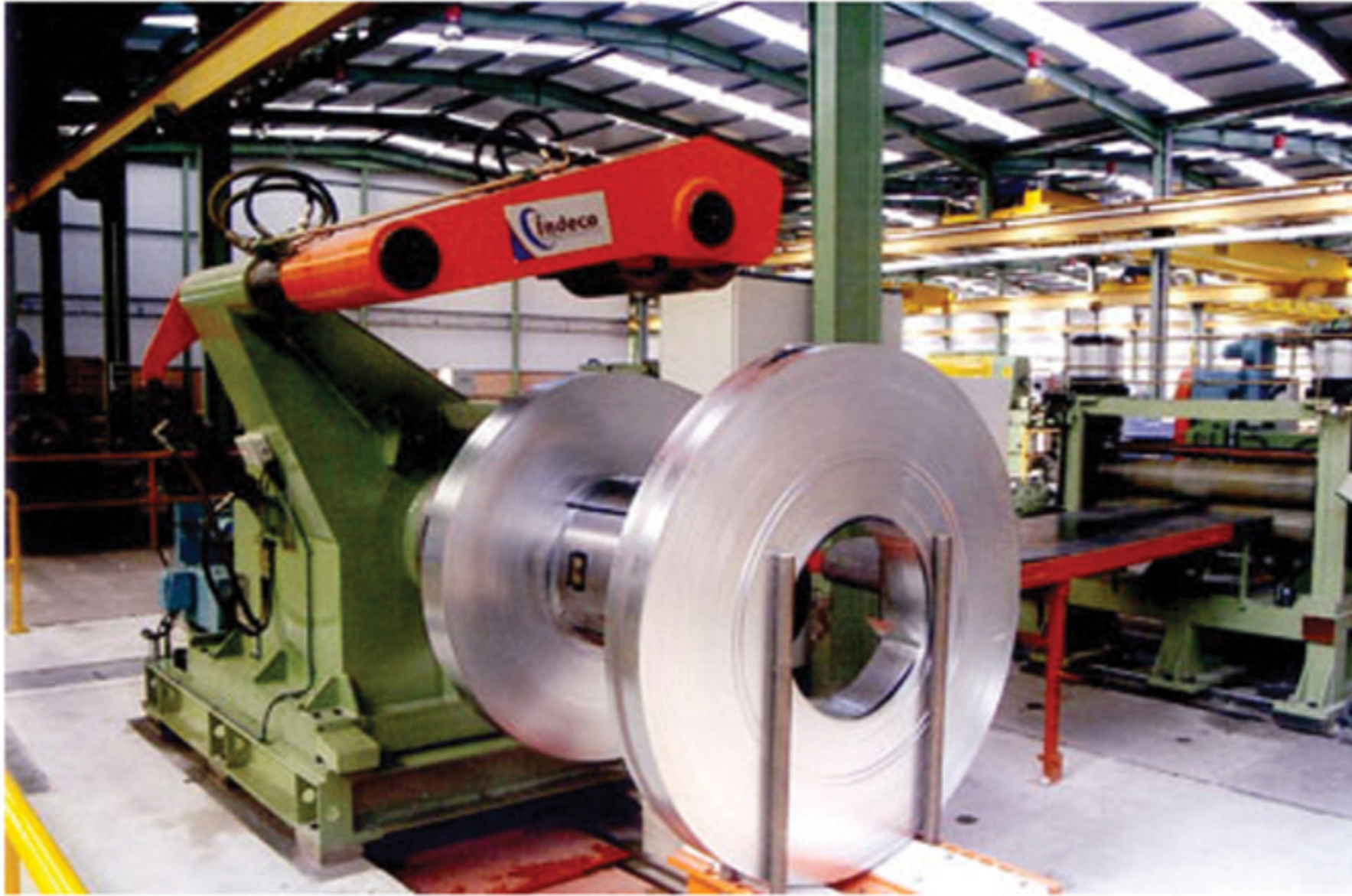
3.- Decoiler with Brake Generator for coils of 1250 mm. width and 15 t. weight.
