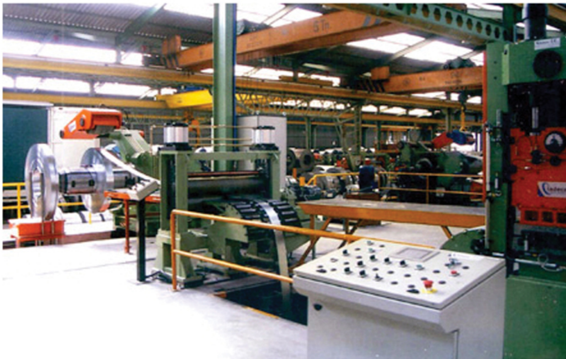
2.- Feeder Rolls for a Cut to Length Line of 0,5 mm. to 2 mm. x 1250 mm.
