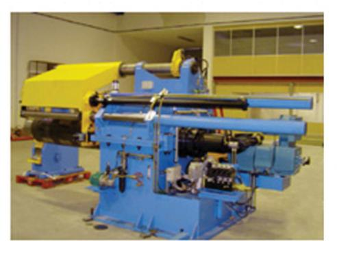
The rewinding system is designed to achieve evenly wound coils with uniform tension and allowing additional roll banding and removing the slit coils without delay.
